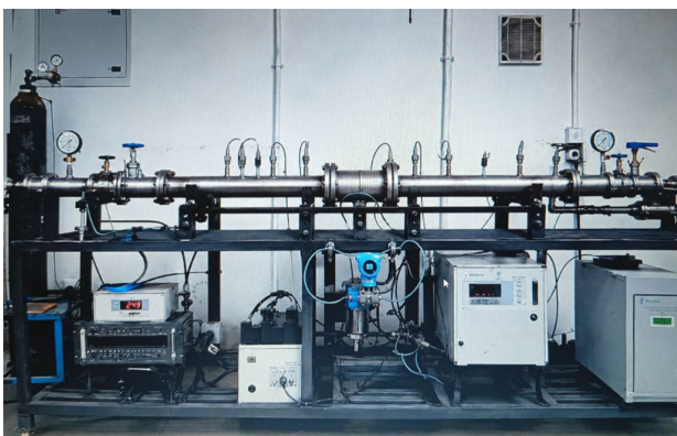
Figure 1. Experimental set up for Joule-Thompson effect.
