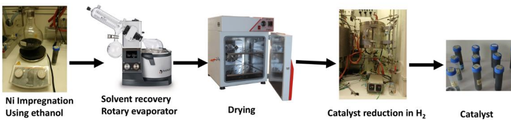
Figure S 1: Work flow of Ni impregnation followed by reduction.
