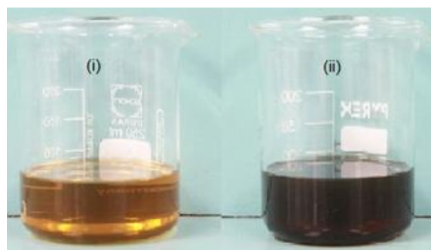
Figure 6. Comparison of tar solution from the gasification of Ni-loaded OPMF (i) and unloaded-OPMF (ii) at 900 °C
