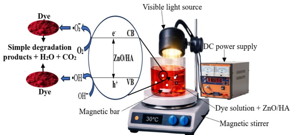
Figure 1. Photoreactor setup for dye solution degradation.
