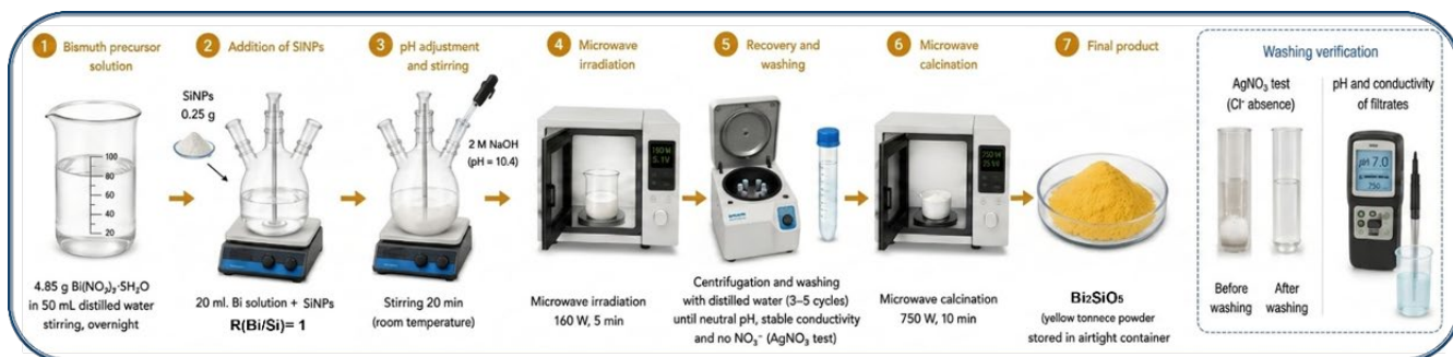
Figure 1. Schematic mechanism of the ultra-fast microwave-assisted solid-state synthesis of monocrystalline Bi 2 SiO 5 using natural sand-derived SiNPs.
