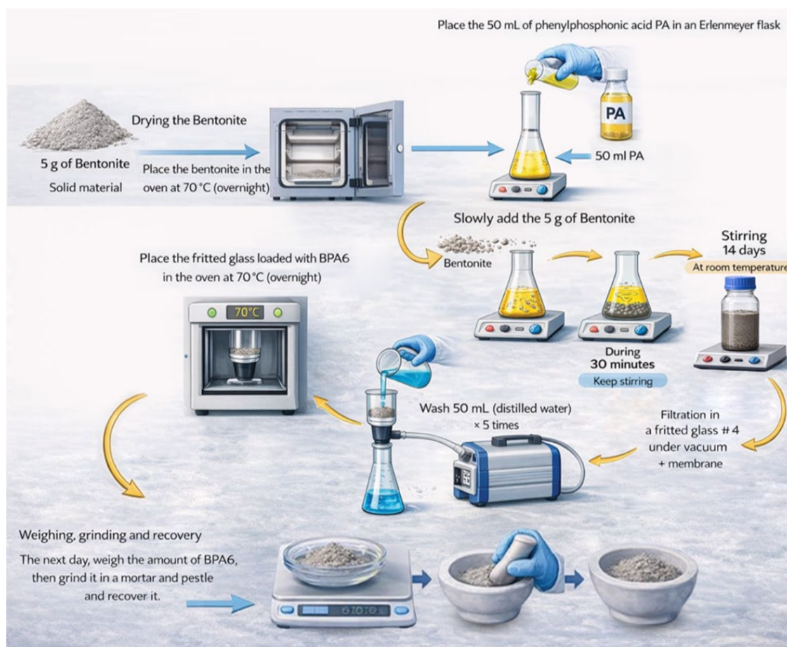
Figure 1. Schematic representation of the synthesis of phenylphosphonic acid–intercalated bentonite.
