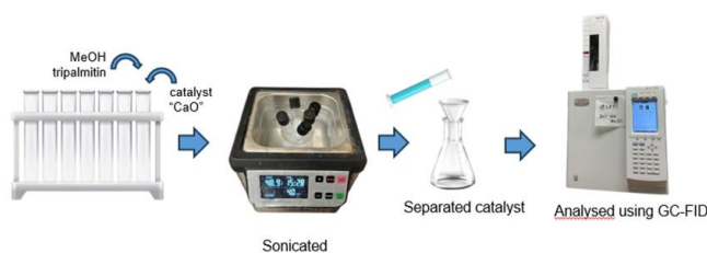
Figure 1. A schematic diagram of the ultrasonic-assisted transesterification setup.
