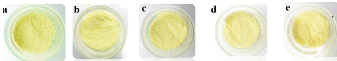
Figure 1. The synthesized bismuth oxide powders: (a). 1 hour of calcination, (b). 2 hours of calcination, (c). 3 hours of calcination, (d). 4 hours of calcination, e. 5 hours of calcination.
