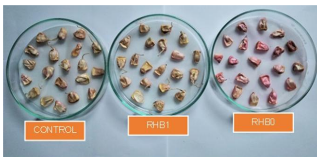
Figure 8. Toxicity test based on corn seed germination using different treatments: Control (distilled water), RHB1 (after photocatalysis), and RHB0 (before treatment).
