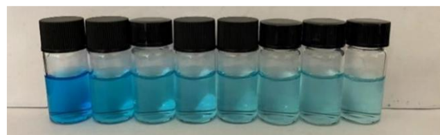
Figure 11. The collection of degraded methylene blue samples every 20-min interval under visible-light irradiation (300 W) for 2 h.
