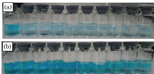
Figure 5. Decolorisation of Methylene Blue after degraded by (a) Gunningite and (b) Wurtzite.
