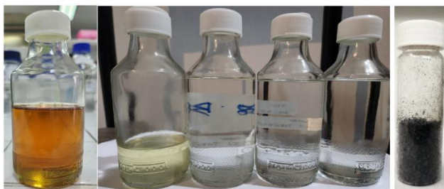
Figure 4. Used cooking oil feedstock (left) and biohydrocarbon produced from different catalyst composites (left to right): NiMo/ \gamma - \text{Al}_2\text{O}_3 , NiMo/ \gamma - \text{Al}_2\text{O}_3 75%-ZAT25%, NiMo/ \gamma - \text{Al}_2\text{O}_3 75%-ZAB25%, NiMo/ \gamma - \text{Al}_2\text{O}_3 75%-ZAL25%, and Biochar.
