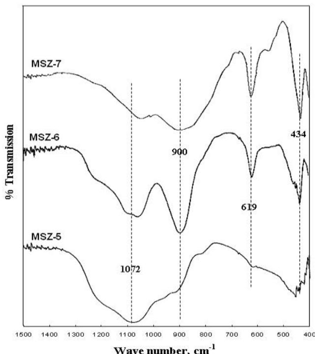
Figure 2: FT-IR spectra of MSZ series of catalyst samples
