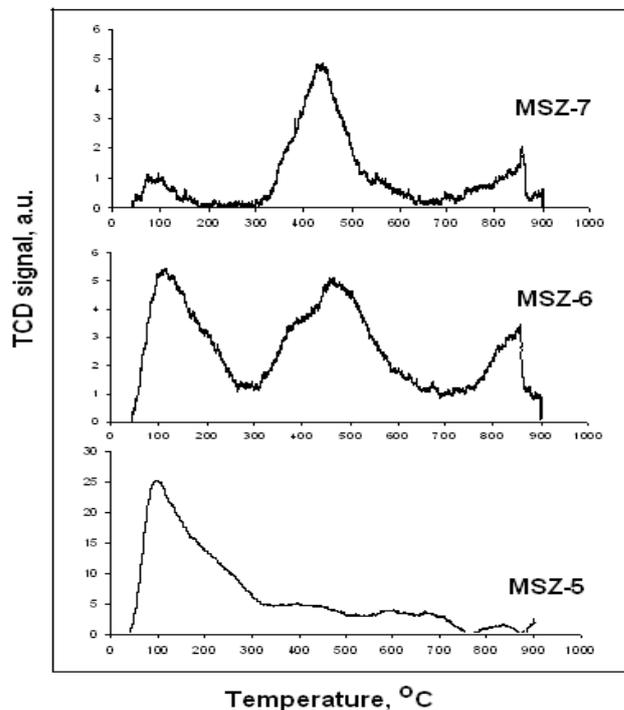
**Figure 4:** NH<sub>3</sub>-TPD profiles for calcined catalyst
