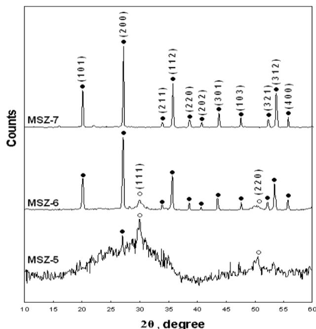
**Figure 1:** XRD pattern of calcined samples: (○) lines due to  $\text{ZrO}_2$  phase; (●) lines corresponds to  $\text{ZrSiO}_4$  phase
