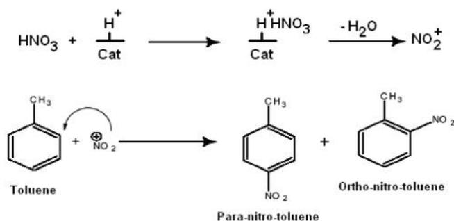
Scheme 2: The plausible reaction mechanism of nitration of toluene over MSZ series of catalysts
