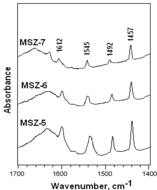
Figure 5: FT-IR spectra of pyridine adsorbed catalyst samples
