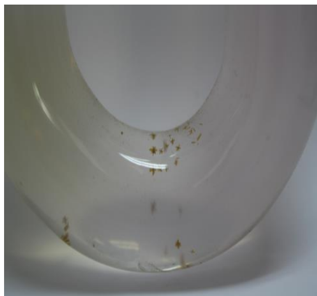
Figure 3. Crystal growth of cobalt (II) oxalate using U-tube method
