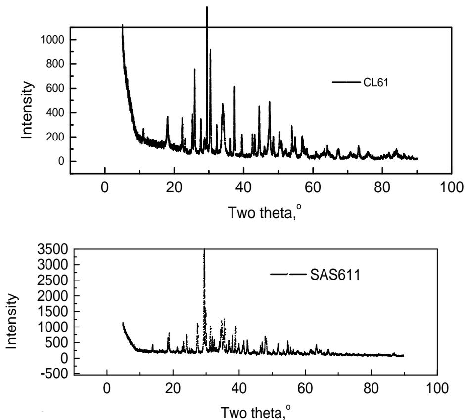
**Figure 2.** (c) The XRD pattern of the samples of sodium aluminum silicate and calcium lanthanum oxide prepared by solid-solid fusion method with different mol ratio of Na:Al:Si (SAS611) and Ca:La (CL61).
