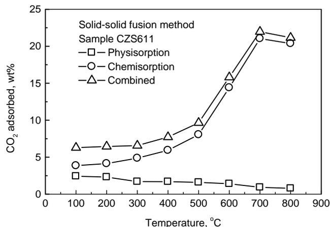
Figure 7. The temperature profile of captured CO<sub>2</sub> by the sample CZSF611 of calcium zirconium silicate prepared by solid-solid fusion method
