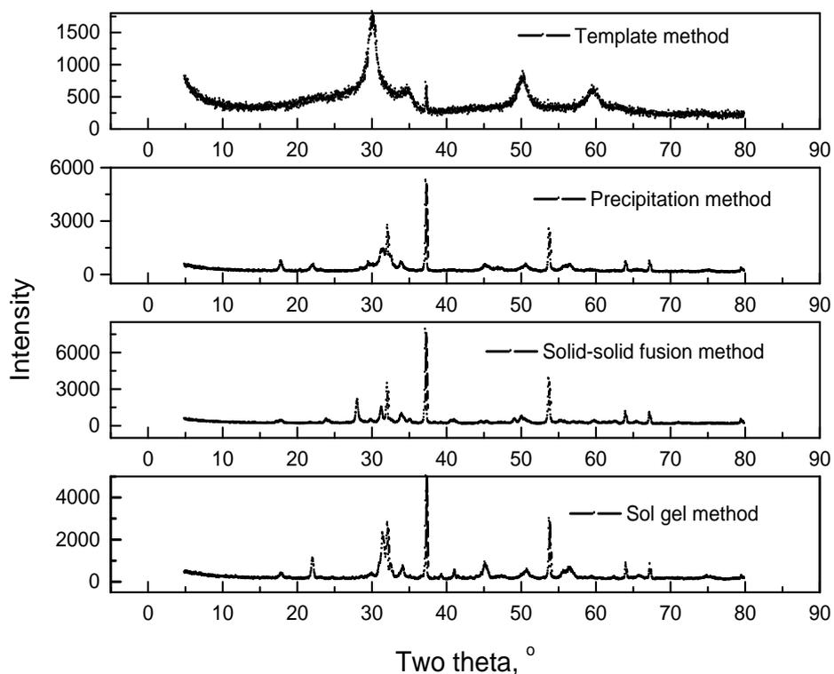
**Figure 2.** (a) The XRD pattern of the samples of calcium zirconium silicate prepared by different methods such as solid-solid fusion, precipitation, sol gel and template methods
