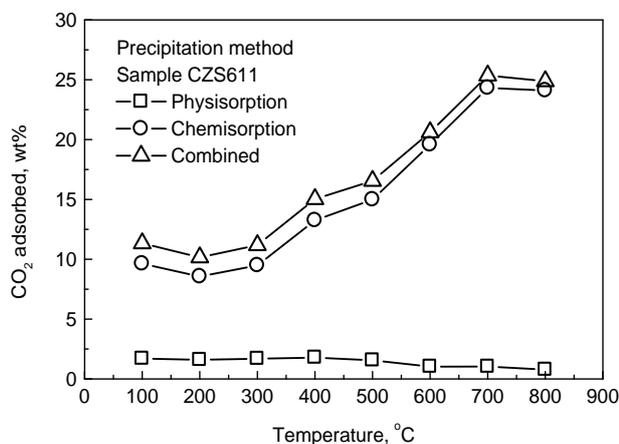
Figure 8. The temperature profile of captured CO<sub>2</sub> by the sample CZSP611 of calcium zirconium silicate prepared by precipitation method
