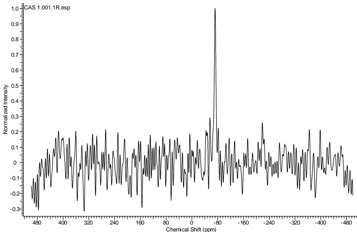
**Figure 4.** (a)  $^{29}\text{Si}$  NMR of the sample CZSF611 of calcium zirconium silicate prepared by solid-solid fusion method; (b)  $^{29}\text{Si}$  NMR of the sample CASF611 of calcium aluminium silicate prepared by solid-solid fusion from calcium oxide, aluminium oxide and silica oxide
