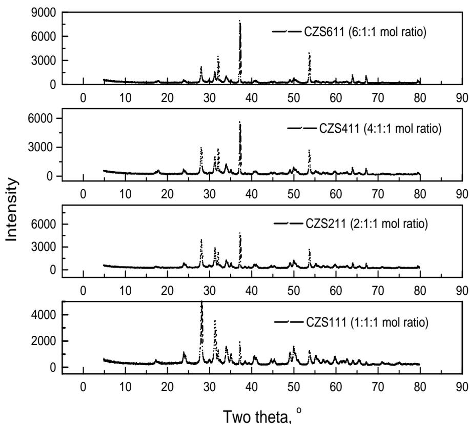
**Figure 2.** (b) The XRD pattern of the samples of calcium zirconium silicate prepared by solid-solid fusion method with different mol ratio of Ca:Zr:Si
