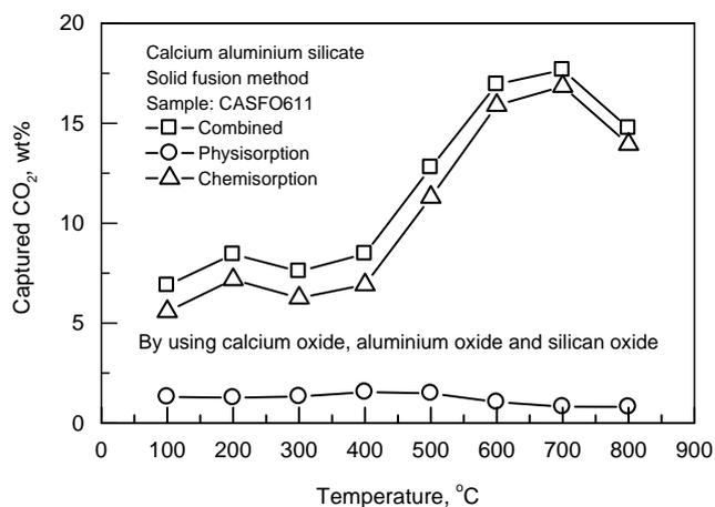
**Figure 13.** (a) The temperature profile of captured CO<sub>2</sub> by the sample CASFNH611 of calcium aluminium silicate by using calcium nitrate, aluminium nitrate and silicon oxide; (b) The temperature profile of captured CO<sub>2</sub> by the sample CASFO611 of calcium aluminium silicate by using calcium oxide, aluminium oxide and silicon oxide
