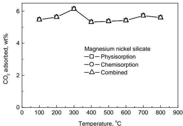
**Figure 14.** (a) The temperature profile of captured CO<sub>2</sub> by the magnesium oxide; (b) the temperature profile of captured CO<sub>2</sub> by the sample MNSF611 of magnesium nickel silicate
