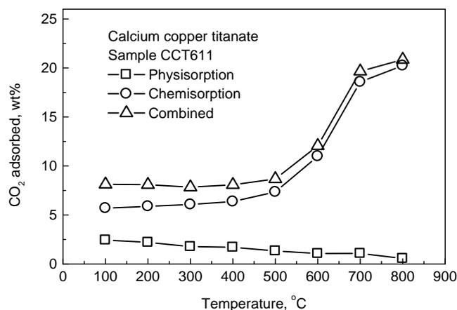
Figure 11. The temperature profile of captured CO<sub>2</sub> by the sample CCTF611 of calcium copper titanate
