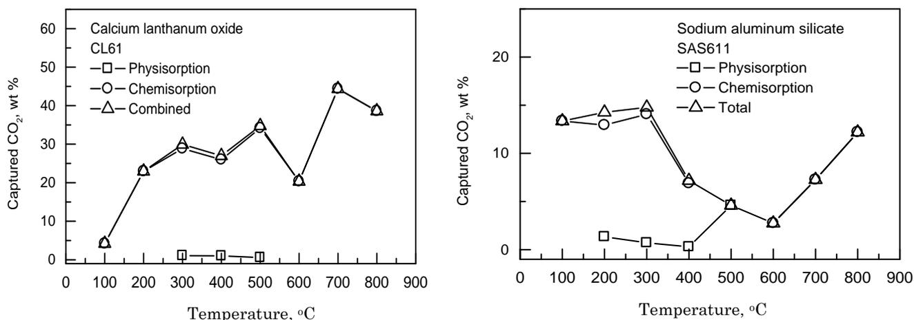
Figure 15. (a) The temperature profile of captured CO<sub>2</sub> by the sample of CL61 of calcium lanthanum oxide; (b) The temperature profile of captured CO<sub>2</sub> by the sample of SAS611 of sodium aluminium silicate
