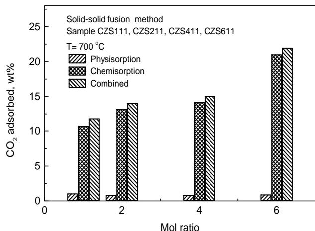
Figure 5. The profile of captured CO<sub>2</sub> by the sample of calcium zirconium silicate prepared by solid-solid fusion method with variable mol ratio
