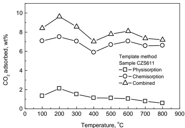
Figure 10. The temperature profile of captured CO<sub>2</sub> by the sample CZST611 of calcium zirconium silicate prepared by template method
