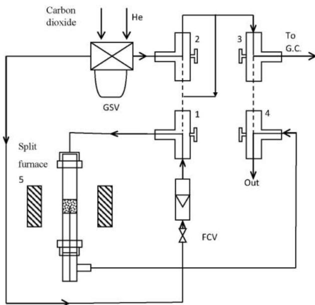
Figure 1. The schematic presentation of CO<sub>2</sub> capture and conversion to syn-gas
