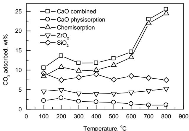
Figure 6. The temperature profile of captured CO<sub>2</sub> by the CaO, ZrO<sub>2</sub> and SiO<sub>2</sub>
