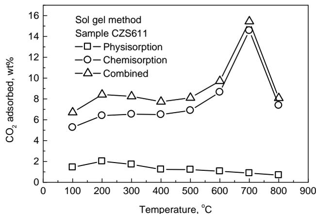
Figure 9. The temperature profile of captured CO<sub>2</sub> by the sample CZSG611 of calcium zirconium silicate prepared by sol-gel fusion method
