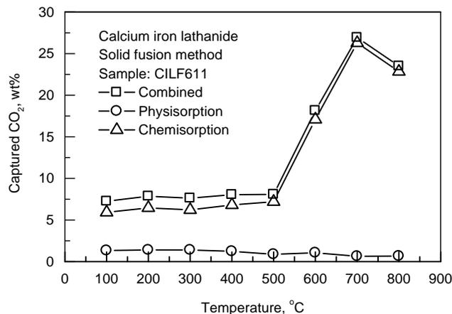
Figure 12. The temperature profile of captured CO<sub>2</sub> by the sample CILF611 of calcium iron lanthanide
