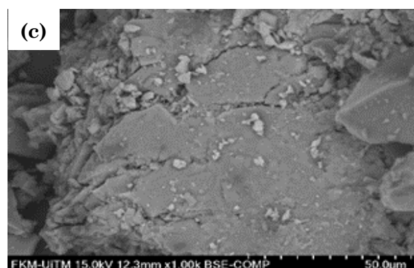
Figure 24. SEM image for precipitate formed from mixing solution of 940Si:900Mg in (a) Test condition 1 (b) Test condition 2 and (c) Test condition 3.
