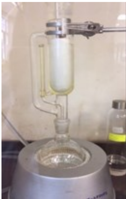
Figure 2. The experimental setup of the Soxhlet extraction method.
